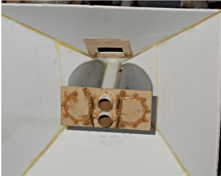
**Chute cannon assembly fitted to airframe. Plenty of epoxy around the top to seal to the airframe and onto the motor tubes for strength. Note also the slot for the electronics tray. Rings around the plywood base are the Kevlar stitching to the chute cannons.**
