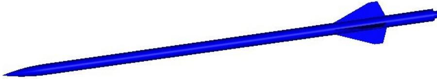
The Rapier is being scratch-built from tubes donated by one of our technicians, which were the cores of Hewlett Packard plotter paper. They are high-quality cardboard, and about 54mm outside diameter, 2 feet long. I wanted to build a rocket capable of taking a RATT I-80 hybrid motor, which is around 30 inches long, but also to be able to fly on a Pro38 solid motor. Thus, a 38mm motor tube was fitted, with through-wall fins, and a 29mm adaptor tube was also built to accommodate the RATT.
