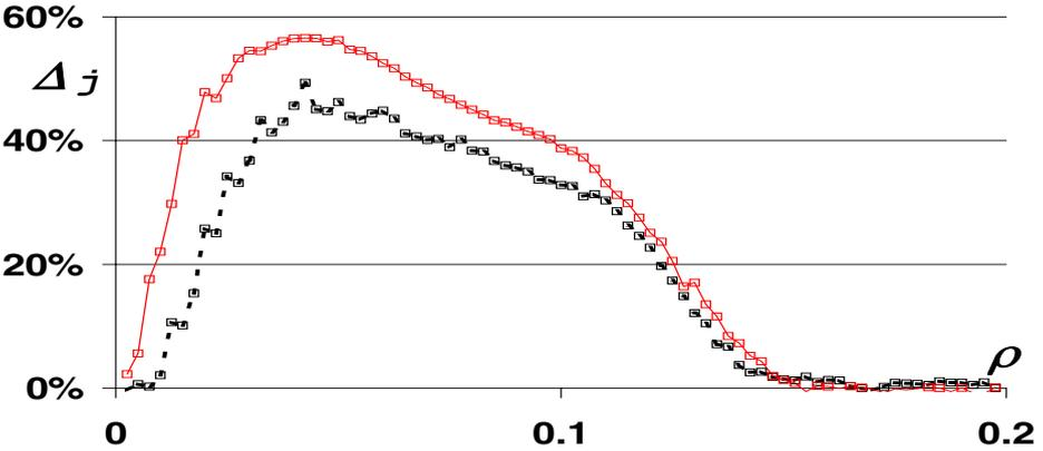
Fig. 4. Relative difference of the flow rates displayed in Fig. 3:  $\Delta j = (J_{\square}/J) - 1$ . Vehicle mixing ratios  $\rho_F/\rho_S \hat{=} 90\% : 10\%$  for lower broken line and  $\rho_F/\rho_S \hat{=} 60\% : 40\%$  for top thin red solid lines.
