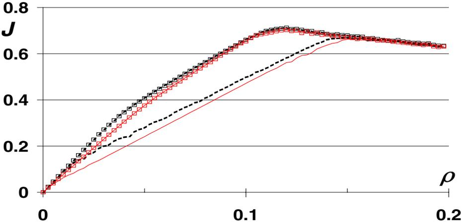
Fig. 3. Same as figure 2 (lower two lines) ( $v_{max,S} = 5$  and  $v_{max,F} = 10$ ) plus additionally scenario ‘□’ with same parameters but slow vehicles now obey no-passing rule (two top lines) thus considerably increasing the flow. Vehicle mixing ratios  $\rho_F/\rho_S = 9/1 \hat{=} 90\% : 10\%$  for black broken lines and  $\rho_F/\rho_S = 3/2 \hat{=} 60\% : 40\%$  for thin red solid lines.
