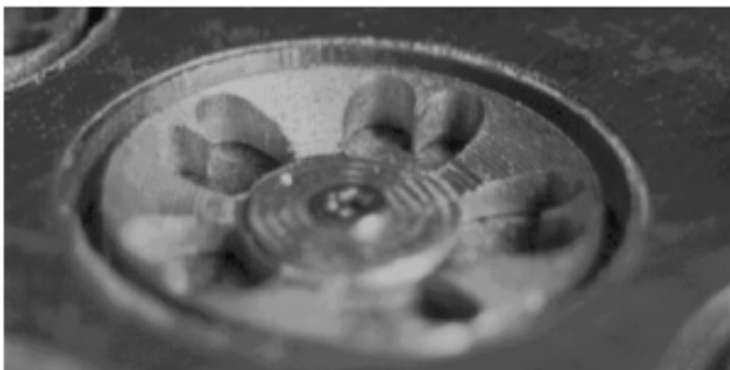
Figure 10: The Spitfire wheel hub insert being cut
