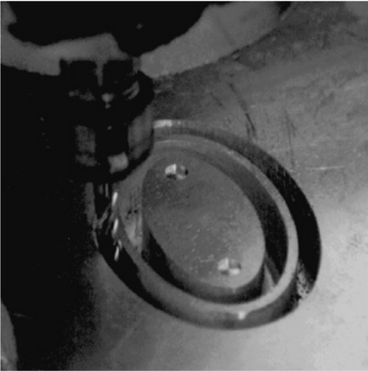
Figure 2: Cutting through 18mm aluminium with a 4mm cutter
