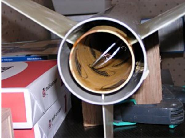
**Fillets on some of the fin joints. Note also the nuts to retain the conformal rail lug**
