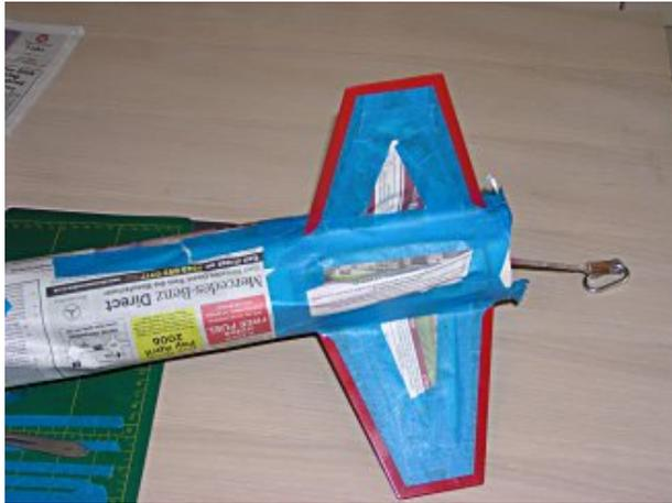
**The fins and airframe masked for the chrome trim, applied over the main colour of red. The stranded steel shock cord (right) was pulled down through the motor tube to hang the rocket for painting**
