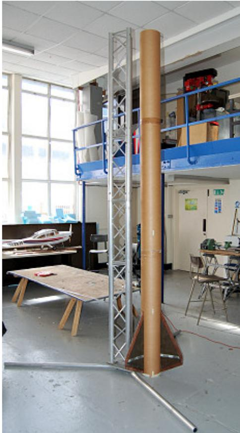
**New launch pad under construction. Sky Streak less nose standing alongside for comparison. Main tower splits into two for transportation, and legs fold. Tilting the pad to load the rocket is also done by folding two of the legs.**
