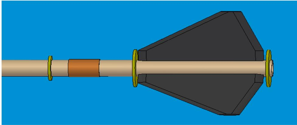
**CAD model of motor mount/fin assembly**
