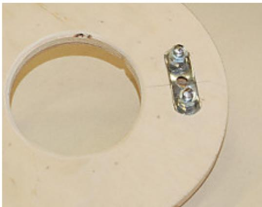
**Back of forward centering ring showing backing plate for U-bolt. Note hole in plate which will take the threaded rod. Thread ends are peened to lock nuts.**
